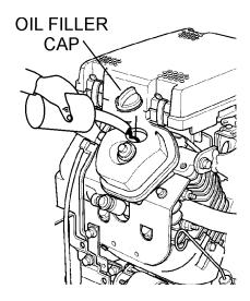
Figure 8. Engine Oil Filler Port
